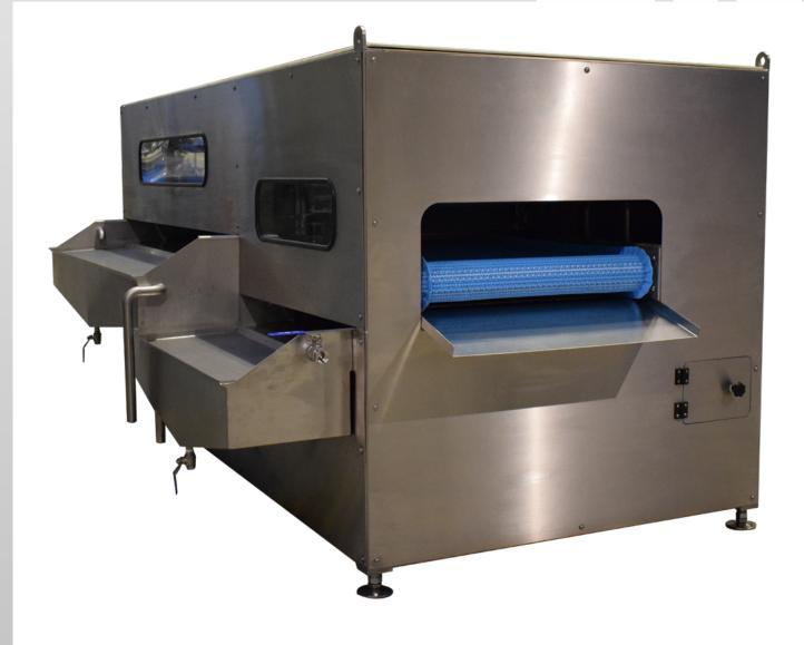
The Normit team developed a solution for blanching flour worms and similar insects, and cooling the product, preparing it for further processing.
