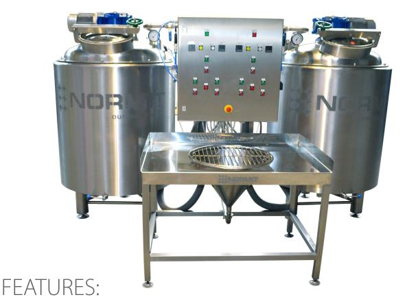
The plant is manufactured entirely from AISI304 stainless steel for the food industry and has teflon scrapers.
