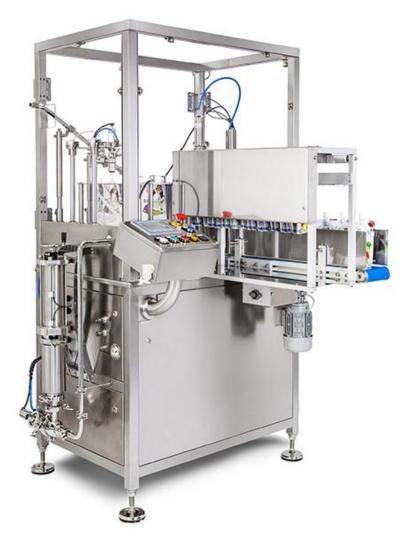
ProfiCut is a complete and versatile work tool that cooks, concentrates, kneads, refines, cuts, mixes, homogenises, pulverises various types of food products.
